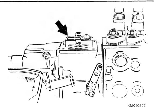
\* Lug cam with torque control
